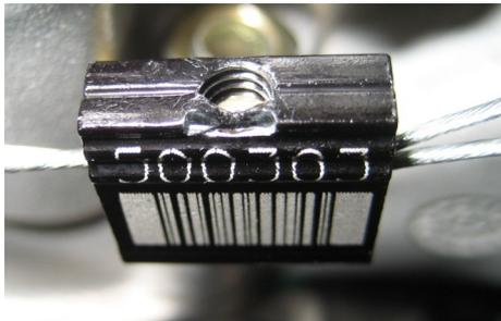
By means of the steel cable the engine must be sealed on one Allen screw (1) of the intake flange, on one stud screw (2) of cylinder and one Allen screw (3) of the cylinder head cover (see attached picture ).
