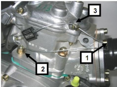
After sealing the engine seal thread must be squeezed using Rotax caliper (part no. 276110).
